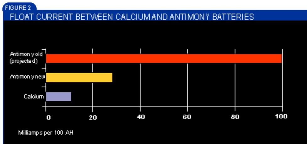
As stated earlier, the VRLA battery is very similar to flooded cells. The antimony additives in VRLA batteries cause the float current and gassing to increase as the battery ages. At the end of
