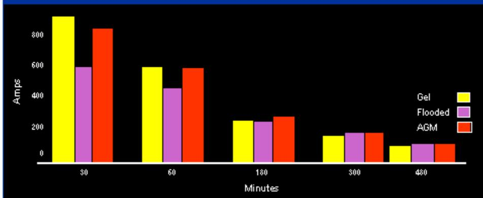
As the data in Table 3 and Figure 1 indicate, the volume of available electrolyte is the critical factor in performance. This means that flooded batteries with lower ampere hour ratings may exhibit better long-rate performance than larger VRLA batteries of either design simply because they have larger acid reservoirs.
